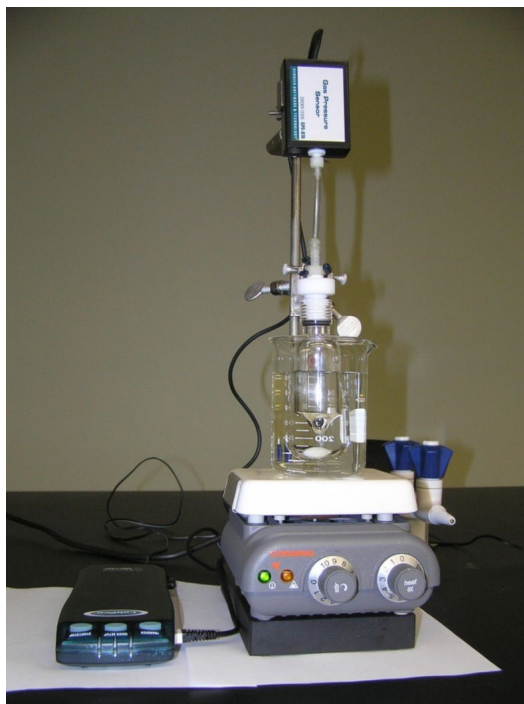
Figure 2: Apparatus for Measuring Catalase-H 2 O 2 Decomposition Kinetics
